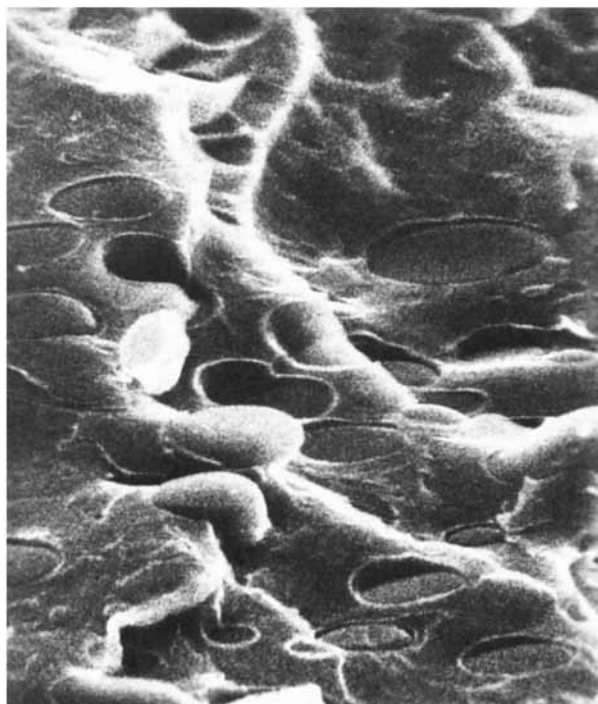
Figure 4 Microphotograph of SEM for 7 : 3 PEMA-PVAc blend (magnification 800).
