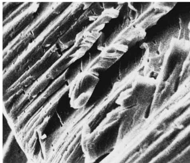
Figure 8 Microphotograph of SEM for 7 : 3 PEMA-PVAc blend and 3% cholesteryl laurate (magnification 800).
