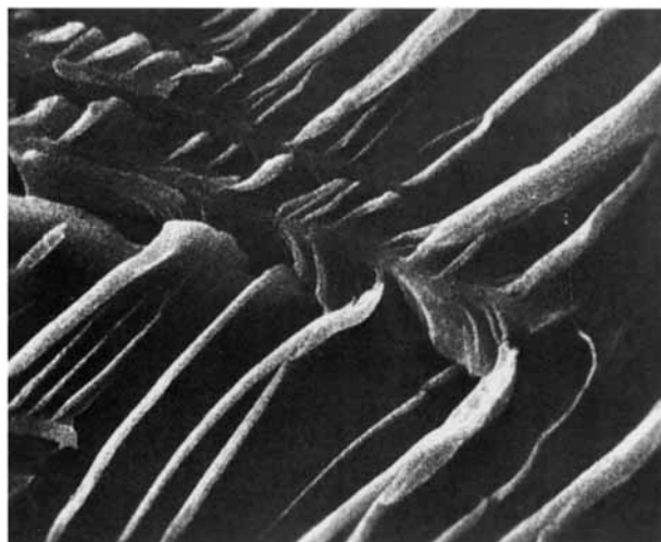
Figure 6 Microphotograph of SEM for 7 : 3 PEMA-PVAc blend and 3% cholesteryl chloride (magnification 800).
