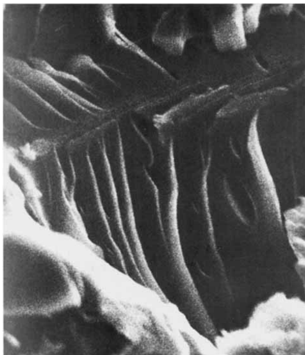
Figure 7 Microphotograph of SEM for 7 : 3 PEMA-PVAc blend and 3% cholesteryl caprylate (magnification 800).
